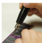
PCB 板迴路修改 Correction of PCB patterns
