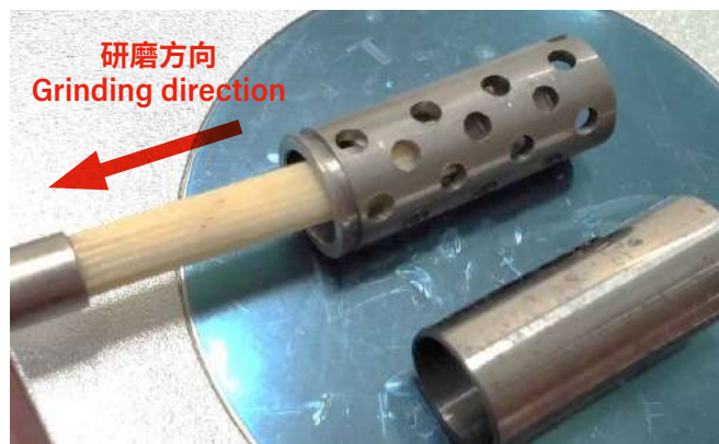
內孔研磨、去毛邊（內孔研磨方向注意） Inner hole grinding, deburring (Pay attention to the direction of inner hole grinding)
